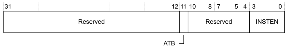
Figure 13-5 TRCEVENTCTL1R bit assignments
